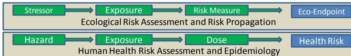
Figure 1: Conceptual model comparing human health risk assessment process to ecological risk assessment process both originally based on EPA risk assessment protocols.
